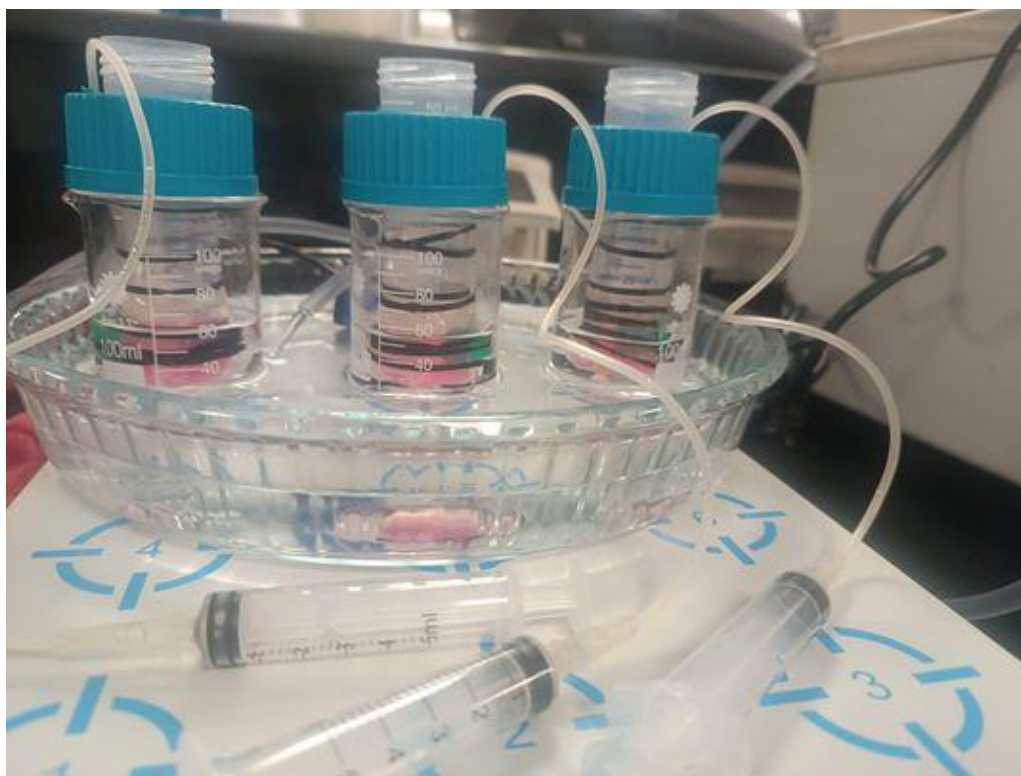
Figure 21 A model system for drug release test
