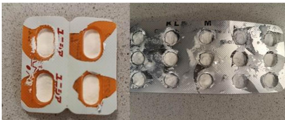
Figure 16 An example of a molding method: a strip into which the first formula was poured.
