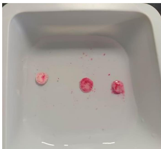
Figure 18 A dish contains S1, S4, and S6 (EC, HPC, and HPMC) was put in SSF at PH 6.8.
